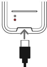
Plug the other end into a USB power source. The red charging indicator illuminates. The green indicator illuminates when the remote is fully charged.
