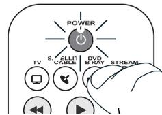
Press and hold the device key you want to program for about 2 seconds, until the POWER key illuminates and stays on. Then release the key.
