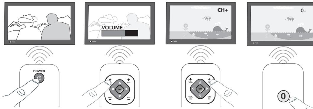
Test commonly used keys with the device (for example, POWER, VOL+, CH+, and 0 for a TV).
