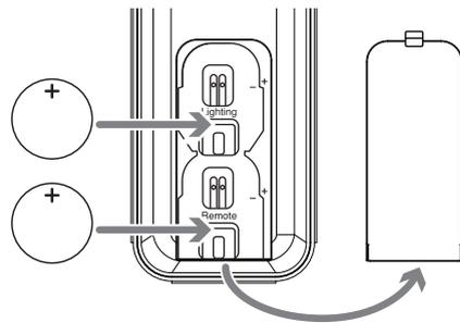
Remove the battery compartment cover, insert the provided coin-cell batteries and push each up under the ridge in the compartment with the "+" marking. Replace the cover.
